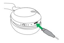
It takes approx. 1 hour and 30 minutes to fully charge. When fully charged, the battery life is 50 hours.
